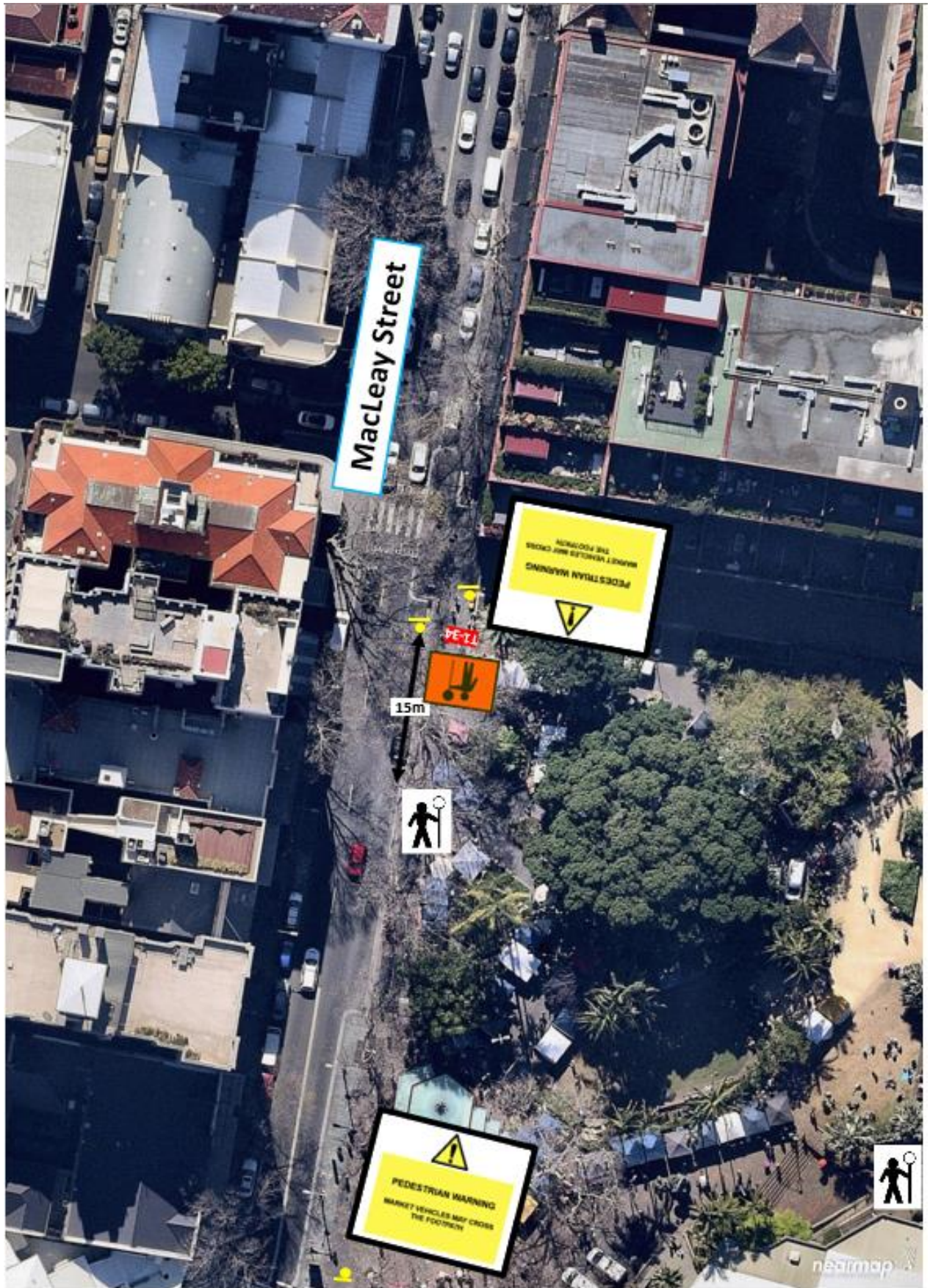
Figure 4-3 Schematic TCP for controlling pedestrian and vehicle conflicts and movements during Bump-in/Bump-out
