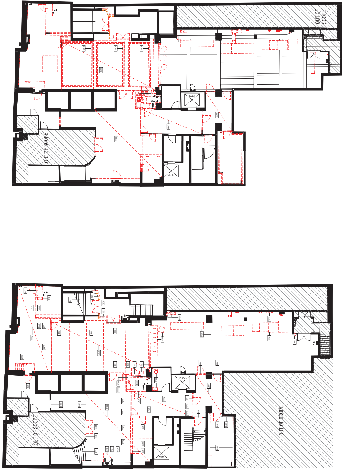
LOWER GROUND EXISTING & DEMOLITION REFLECTED CEILING PLAN
